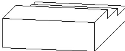
SHED ROOF - Similar to Flat roof except that it has a noted slope in one direction.
