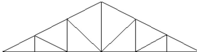
WOOD TRUSS - This is made up of various size lumber or timber such as beams, bars, and ties, usually arranged in triangular units to form a rigid framework and may be flat, shed or pitched. Spans are limited due to the strength of the material.
